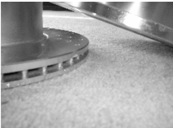
16v 1986 SAAB 900 Aero brake discs shown
